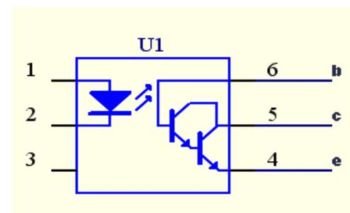
The optional opto-coupler’s output is a Darlington transistor, which gives great flexibility to operation. If needed we might be able to help out with a circuit solution for specific competitor amplifier modules.
