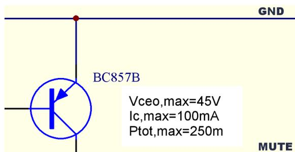
The above schematic shows the mute output circuit. The output needs no glue components if it has to control our own power amplifier modules PA1CC, PA3CC and PA6CC.
